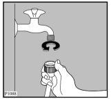
If only a cold water supply is available, connect the two hoses to a cold water outlet by means of a «Y» connection piece.
